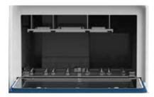
Automatic nucleic acid extraction processing can be performed on 32 samples simultaneously, greatly liberating the hands of researchers
