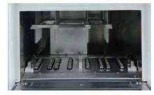
Disposable sheath insulates magnetic rods and samples, and machine is equipped with UV sterilization and air filtration adsorption systems to reject cross contamination
